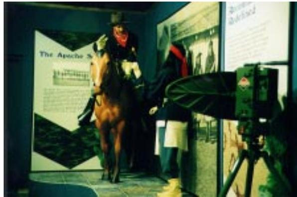
**PPS-5.** Replacing the Indian Scout of a century ago, the three-man Ground Surveillance Radar team gives the maneuver battalion commander a highly mobile, almost all-weather, round-the-clock surveillance of the battlefield. The AN/PPS-5 can detect people moving up to three miles and can spot vehicles at over six miles, making it useful for detecting enemy move-
